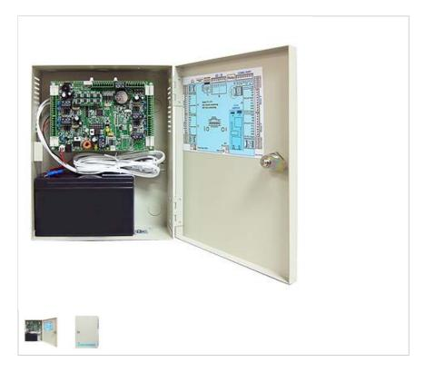
•The PC-1074/T is designed for high-security access control and real-time monitoring environments from medium size to complex multi-site installations.
